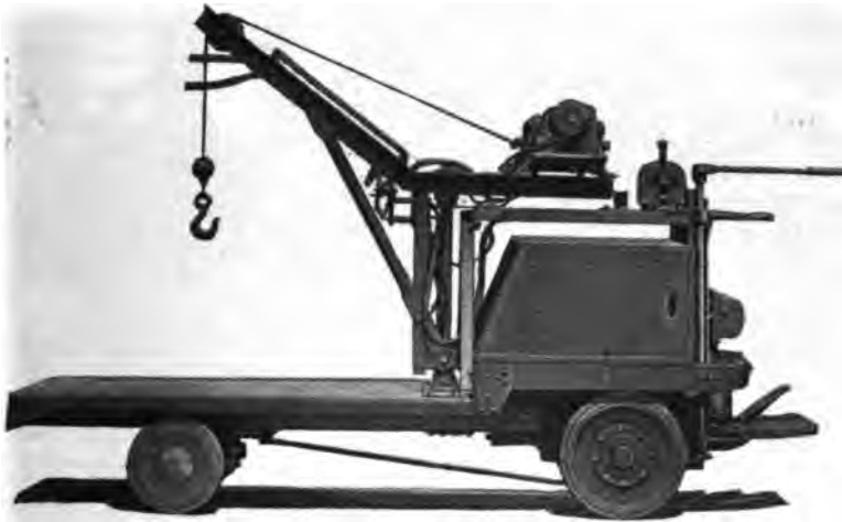
FIG. 3.—4,000-LB. LOW PLATFORM TRUCK WITH 1,000-LB. ELECTRIC SWIVEL CRANE
